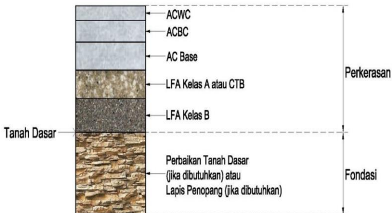
Gambar 2 Detail Perkerasan Lentur Metode Bina Marga 2017
