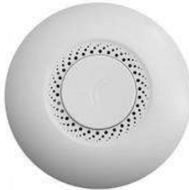
Figure 9. The Wireless Indoor Access Point RBcAP2nD (cAP) is a suitable alternative for use as a CAP
